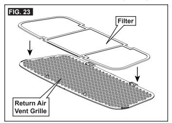
6. Install return air vent grille into the ADB. Slide return air vent grille tab into slot in ADB and rotate up and snap in place. See (FIG. 24).
