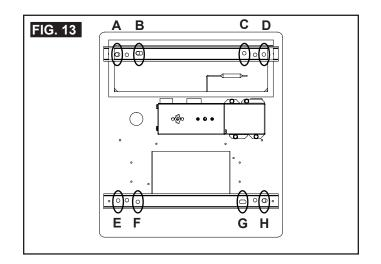
g. **NOTICE** Tighten mounting bolts to correct torque specifications. Overtightening could damage unit's base pan or ceiling template. Not enough torque will allow an inadequate roof seal, and could cause a leak.
