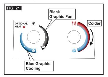
The thermostat controls the compressor On/ OFF operation within a temperature range of approximately 65° F and 90° F measured at the ADB inlet.
