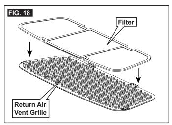
Install return air vent grille into the ADB. Slide return air vent grille tab into slot in ADB and rotate up and snap in place. See (FIG. 18).
