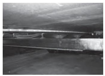
1. Wipe down all exposed mechanical slide components: gears, rails, shafts, etc. Look for any damage, or caked accumulation of grease and dirt. Remove any of this accumulation.
