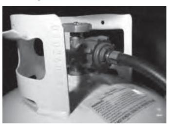
The safety features of this system prevent gas from flowing unless the connection is tight and will limit excessive gas flow. In cases of extreme heat, 240° to 300°F, at the connection, the connection to the cylinder will be shut down.
