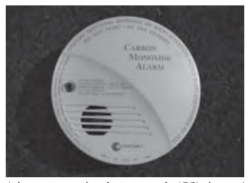
A battery-powered carbon monoxide (CO) detector/ alarm is installed in or near the main sleeping area. Detailed operating and maintenance instructions are in the Owner's Information Packet.
