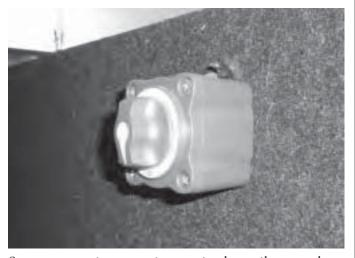
Some accessories or equipment in the trailer may draw small amounts of current even when turned OFF. A battery disconnect (or "load disconnect") system allows you to disconnect the house batteries. Disconnecting
