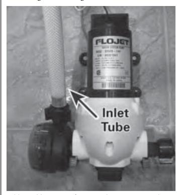
Add potable RV antifreeze to the system. Dutchmen recommends disconnecting the water pump inlet tube and pumping antifreeze from a container into the system.
