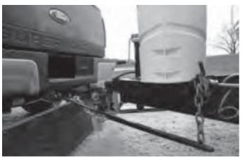
Use a sway control system installed and adjusted according to the sway control manufacturer's instructions.
