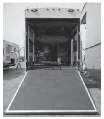
The cargo door/loading ramp gives you complete access to the trailer cargo area. When lowered, the loading ramp allows you to easily load rolling cargo, bicycles, small motorcycles and ATV's, and small vehicles. This section outlines the safety precautions you should take when loading and unloading cargo and vehicles, as well as loading/unloading procedures, techniques and tips.
