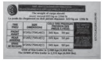
Both placards and certification labels are permanently attached to the trailer on the forward half of the left side, and are easily readable from outside the vehicle without moving any part of the vehicle.
