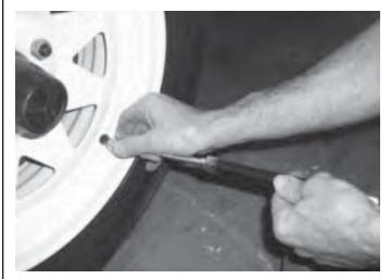
The recommended tire inflation pressure is the proper pressure when a tire is cold. A "cold" tire is one that has not been driven on for at least three hours. When you drive, your tires get warmer, causing the air pressure within them to increase. Therefore, to get an accurate tire pressure reading, you must measure tire pressure when the tires are cold.
