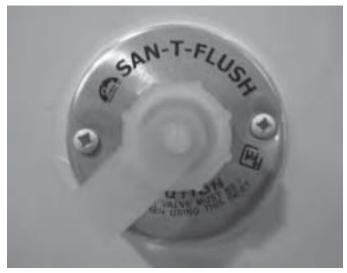
If equipped, the San-T-Flush kit has been installed to rinse the interior of the black tank. Similar to the water fills located on the exterior of the unit, a separate hookup is placed on the exterior.
