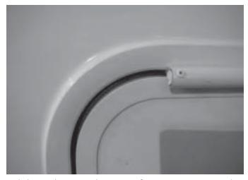
While washing, make note of any maintenance that may be needed. Closely inspect the sealants around roof accessories (vents, antennas, racks, etc.), windows and doors. Reseal as necessary before winter rains or snows accumulate.
