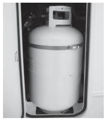
1. Before removing an empty cylinder for refilling, close the main valve on the empty cylinder – hand tighten only. Rotate the changeover lever on the regulator so that it points to the full cylinder.
