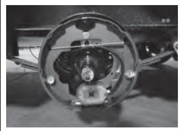
Your trailer is equipped with electric brakes. They are similar to the drum brakes in many trucks and cars. The basic difference is that rather than using hydraulic pressure for activation, your trailer brakes are actuated by an electromagnet.
