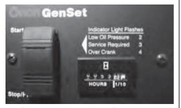
See the generator Operating Guide in your Owner's Package for complete operating and maintenance instructions. The generator control panel features:
