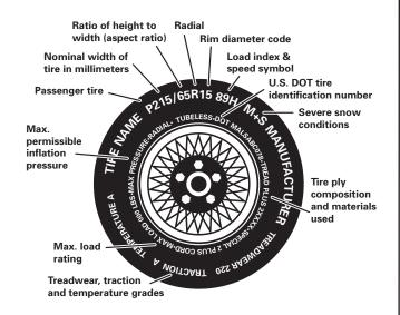
P - The "P" indicates the tire is for passenger vehicles. NOTE: Passenger car tires are not recommended for use on trailers.
