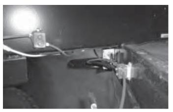
Be careful to prevent damage to the 7-way cord. When hitching and unhitching, make sure the cord is out of the way and cannot be damaged by the hitch and/or pin box. Do not allow the cord to drag on the ground. When not in use, cover the cord connector to prevent moisture from entering the connector. Clean the contacts in the cord with a contact cleaner every six months.
