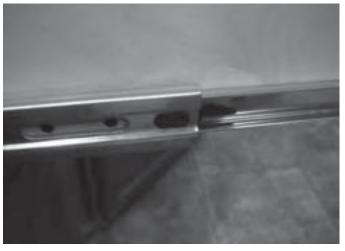
The drawers run in metal guides. To remove a drawer, pull it out until it stops. On each side of the drawer is a latching mechanism. Press the latch while pulling the drawer out slightly to clear the latch tab (ball bearing drawer guides only). Pull the drawer out and lift slightly to clear the guide wheels.
