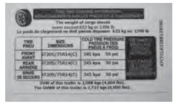
The other is the tire and loading information tag. It shows the size of the tires originally installed on the trailer or the tires that are standard for these trailers, the recommended cold tire inflation pressure, cargo weight capacity of the trailer and the trailer VIN.
