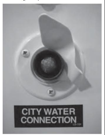
The city water system is connected through a potable water hose to a hookup on the exterior wall of the trailer. Since campground water systems have varying pressures, a pressure regulator should be used to reduce the city water pressure to the trailer. Because the connection is pressurized, there is no need to use the water pump.
