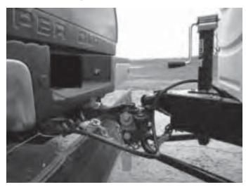
10. Connect the 7-way power cord to the tow vehicle receptacle and the breakaway switch lanyard to a non-removable part of the hitch or the tow vehicle chassis.
