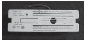
A propane leak detector is mounted near the floor. It is powered by the trailer 12-volt DC system. The detector senses the presence of propane and some other hydrocarbons. If propane is detected, the alarm will sound. The detector will not automatically shut off the propane system.
