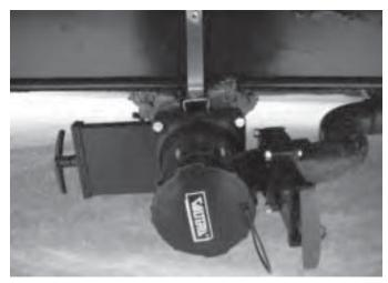
Drain the holding tanks only when they are at least 3/4-full. If necessary, fill the tanks with water to 3/4-full. This provides sufficient liquid to allow complete flushing of waste material into the sewer line.
