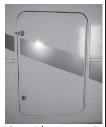
A firm tug on the door at the opposite corner from any binding can almost always eliminate this problem. Another technique is to use a mallet and block of wood to remove any slight interference. During the course of ownership, these doors might normally require this minor routine maintenance adjustment, and is not a warranty defect.
