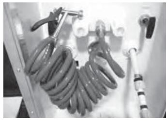
Disconnect the outside shower hose (if equipped) and drain the hose. After all water is drained from the hose, reconnect hose.
