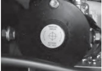
This system uses a hydraulic cylinder and a pump to push the slide room in and out. The system is activated by using a remote control device. As with the other slide mechanisms, it is possible to retract the room manually by installing an electric and/or battery driver into the socket on the pump and manually driving the pump. The pump will be driven clockwise for extend and counter clockwise for retraction.
