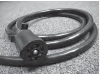
Be sure the breakaway switch activating pin is secure in the switch. Coil and stow the 7-way power cord.
