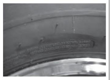
The tire manufacturer's recommended inflation pressure is stamped on the sidewall of the tire. The maximum tire pressure is also listed on the trailer VIN label. Check the tires frequently to be sure they are properly inflated. Always check tire pressure when the tires are cold. Check that the air pressure is equal in all tires. When replacing tires, make sure the replacement tire is the same size and load capacity as the original. See the "Tires and Wheels" chapter for more information.
