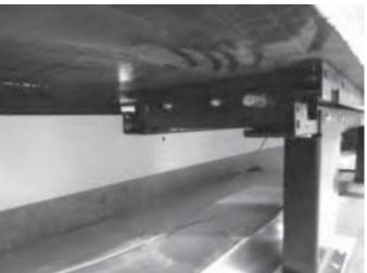
The Happi-Jac electric above floor slide system can be extended or retracted manually using a 3/4" socket and ratchet tool. To retract the room, remove the access panel generally located below the sofa or dinette seat. Place the socket on the shaft connected to the motor and gear mechanism and turn clockwise to extend the room or counter clockwise to retract it. Once the room is retracted it is advisable to secure the room in with travel locks.
