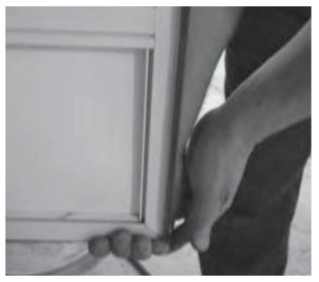
Normal operation and over the road dynamics will cause the screen door hinges to settle slightly, causing the screen frame to drag on the threshold.
