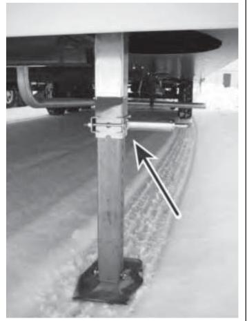
Pull the lock pin on the landing gear leg and allow the drop tube to drop to the ground. Adjust the tube up or down so you can re-engage or re-pin in the nearest adjustment hole.
