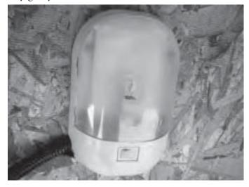
Some interior storage areas may be equipped with 12-volt lights. Be sure these lights are OFF when you close the door or your battery could be rapidly discharged if you are not connected to shore power.
