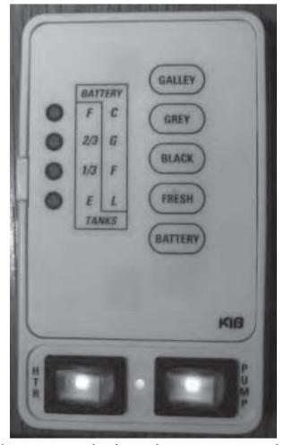
The monitor panel is designed to give approximate liquid levels of the fresh, gray and black water tanks at a given moment as well as a charge value (based on voltage) of the battery.
