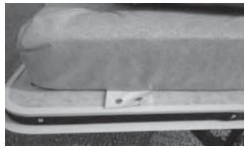
• From the inside remove the mattress from its storage position. There are four snaps in the front corners that will need to be released to remove. This will make inserting the bow properly much easier.
