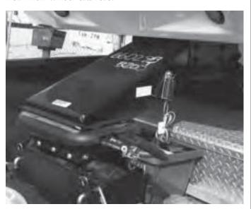
Use a hitch and receiver assembly sized for the 2" SAE king pin and rated to pull not less than the Gross Vehicle Weight Rating of the fifth-wheel trailer. The receiver should be attached to the truck chassis. No weight distributing or sway control devices are needed with a fifth-wheel hitch.
