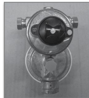
A two-stage regulator performs the pressure reducing function as previously described. This is accomplished in two stages. Two regulators are used in the same body to reduce the pressure of the LP gas in the tanks for use by the appliances in the camper.
