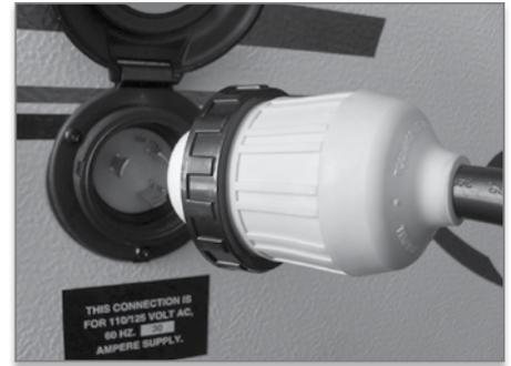
**For models with a removable power cord:** To attach an outside power source, open the cap on the power cord inlet and attach the removable cord provided. The power cord is 25 feet in length, and designed for 30-amp service.
