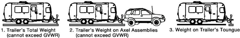
The allowable personal cargo must be distributed in your trailer in such a manner that the Gross Axle Weight Rating is not exceeded.
