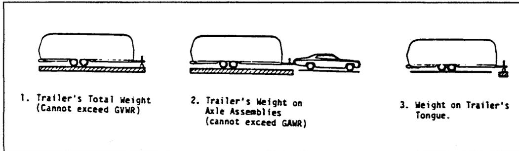
Use a scale, such as a bathroom scale, that has a lower weight limit than your tongue load to check the tongue weight by using the following method (see illustration).
