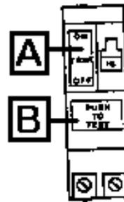
**Important:** If handle B does not move to TRIP position when test button is pressed, the GFCI breaker protection is not complete. If this happens, replace GFCI breaker.
