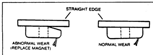
Even if wear is normal is indicated by your straightedge the magnets should be replaced if any part of the magnet coil has become visible through the friction material facing of the magnet. It is also recommended that the drum armature surface be re-faced when replacing magnets. (See Brake Drum Section) Magnets should also be replaced in pairs (both sides of an axle). Use only genuine Dexter replacement parts when replacing your magnets.
