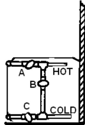
Open the hot side of the galley or lavatory faucet and turn on the water pump switch located on the monitor panel. For some time the open faucet will only sputter. This is because the water heater is being filled and air is being pushed out through the lines. Once the water heater is full a steady stream of water will come from the faucet. Now open a cold faucet. It will sputter for a short time, but will soon expel a steady stream. All other faucets can now be opened until all air is expelled.
