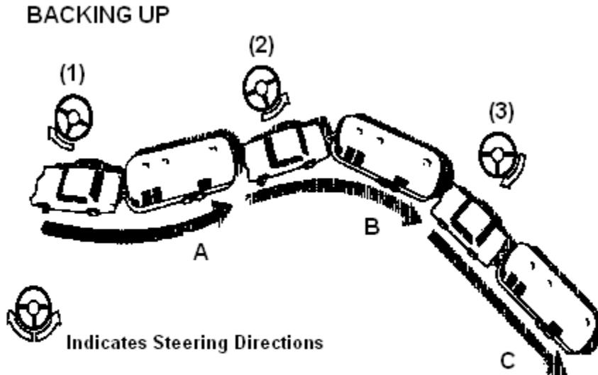
Position (A) start. Turning steering wheel as shown in (1) will put you in trailer position (B). Turning steering wheel shown in position (2) puts you in trailer position (C). Steering position (3) returns front wheels for straight backing.
