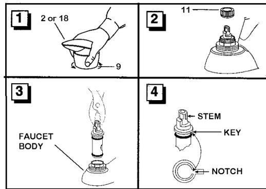
4. To reassemble, reverse the previous steps. Turn the cartridge stem to ON position, so that the hole in the piston lines up with the hole in the outer shell. Push the cartridge straight down into the body making sure the key on the cartridge fits into the notch in the body. This will correctly position the cartridge. Replace the cartridge nut, start by hand, **DO NOT CROSS THREAD**, and tighten firmly.
