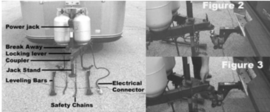
A low hitch ball increases tail wagging tendencies by lowering the nose of the trailer, thus changing the center of support for the trailer and reducing the weight on the four wheels of the tow vehicle. With proper hitch installation and hitching up, the bar should have a noticeable amount of the deflection or bending. A little practice with your rig will teach you how far to pull the bar; you may wish to mark the chain links that match your rig.
