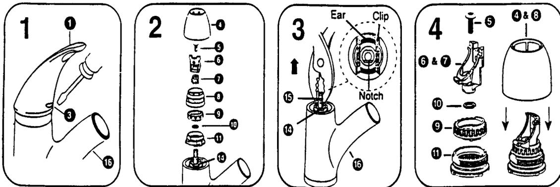
**Open faucet handle to relieve water pressure and ensure that complete water shut-off has been accomplished.**
