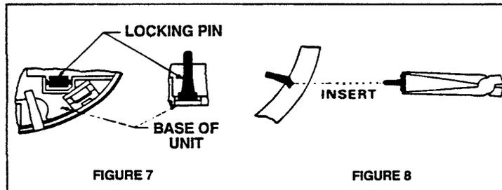
1. Remove the breakaway locking pin from the unit by rocking pin back and forth.
