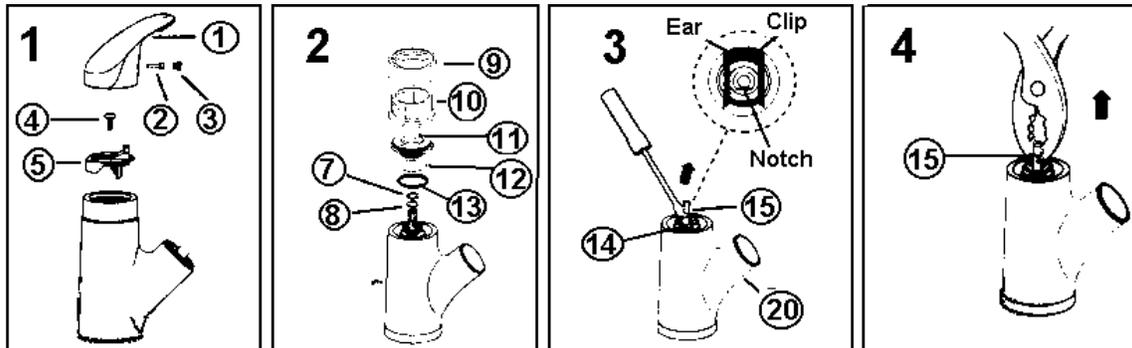
**CAUTION:** Always turn water OFF before removing existing faucet or disassembling the valve. Open faucet handle to relieve water pressure and ensure that complete water shutoff has been accomplished.
