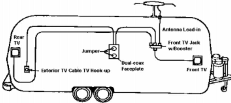
COAXIAL CABLE WITH SATELLITE ANTENNA
