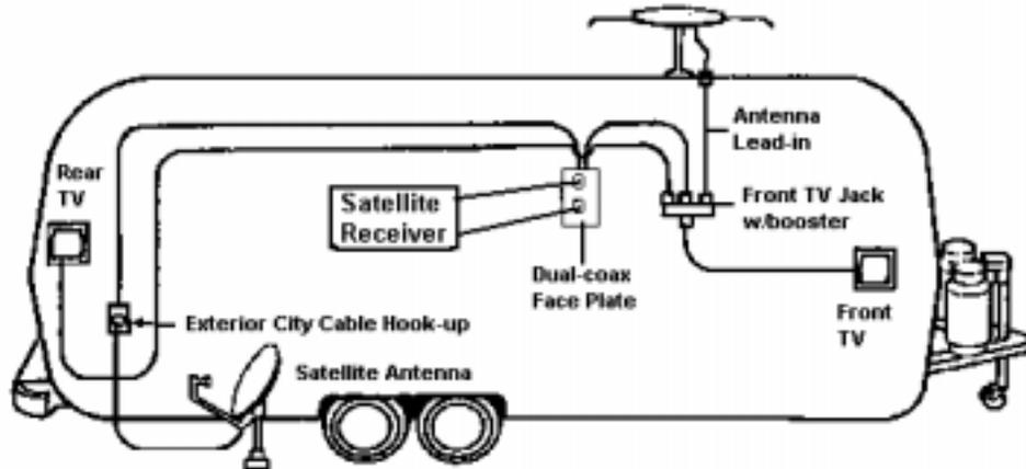
**SATELLITE ANTENNA WIRING**
