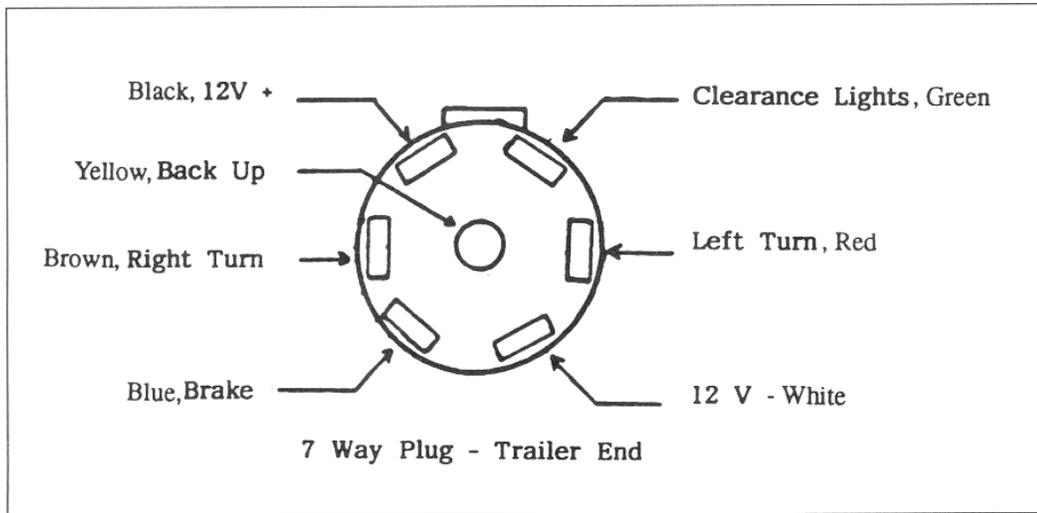
**Note:** The 7 way wire is spliced to the main harness in the front of the trailer.
