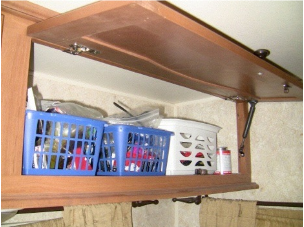
RV Overhead Storage Bins with Gas Lifts Showing
