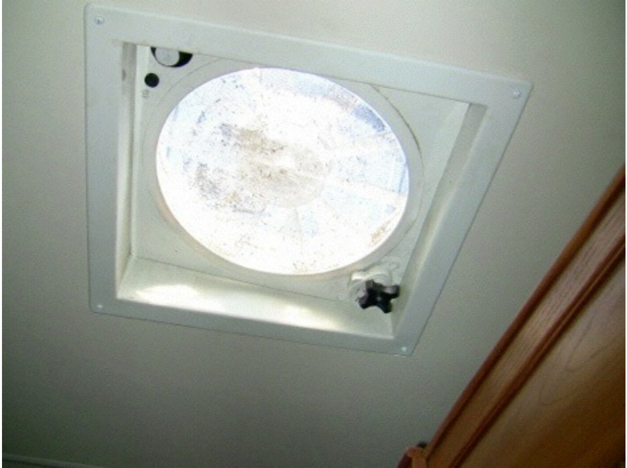
RV Super Fan Kitchen Vent – unfortunately with small bits of insects and dirt shown.
