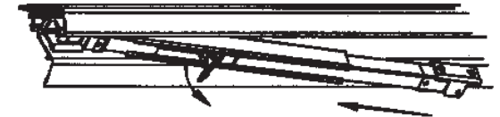
Unlock flipper latch slide arm outward
