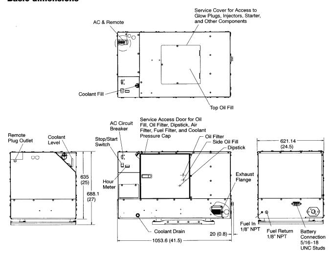
**Note:** This outline drawing is provided for general reference only and is not intended for design or installation. For more information see Operation and Installation manuals or obtain 500-4040 drawing and wiring diagram from your distributor/dealer.
