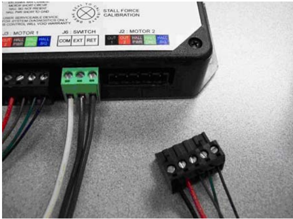
Motor connection at board
