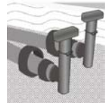
Fig. 8.7 Low point drains
