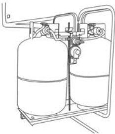
Fig 7.7 Two propane cylinders
