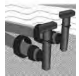
Fig. 8.7 Low point drains
