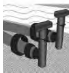
Fig. 8.7 Low point drains
