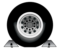
Properly Chocked Wheel
