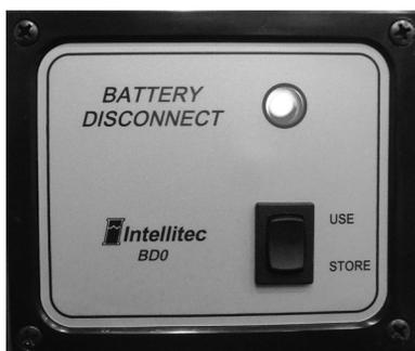
When the switch is turned to USE (on) and the trailer is plugged into a 110-volt shoreline, the 12-volt distribution panel will receive power from the converter and the batteries will be charged through the converter charging system.
