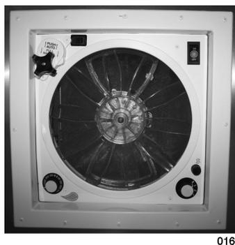
The optional high-volume roof vent system is designed to quickly exhaust stale, hot air and draw in fresh air. It is great to use when the outside temperature does not call for air conditioning, but heat has built up in your coach.
