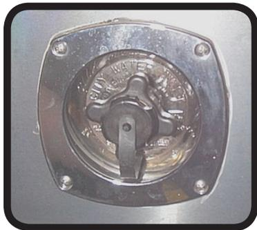
To reassemble, rotate the inlet side of the strainer until stops are felt. The "O" ring performs the sealing and too much pressure will only break the strainer.
