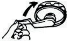
Turn elevating crank in “UP” direction until some resistance to turning is noted. Antenna is now in operating position.
