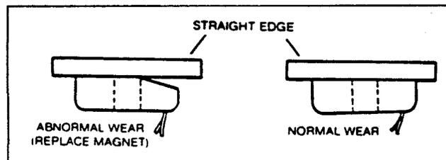
Even if wear is normal as indicated by your straightedge the magnets should be replaced if any part of the magnet coil has become visible through the friction material facing of the magnet. It is also recommended that the drum armature surface be re-faced when replacing magnets. (See Brake Drum Section) Magnets should also be replaced in pairs (both sides of an axle). Use only genuine Dexter replacement parts when replacing your magnets.
