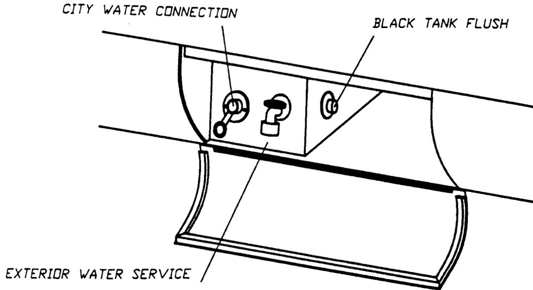
The city water hook-up is found on the lower roadside of the trailer in the utility compartment. A short piece of hose has been provided to extend the city water hookup.
