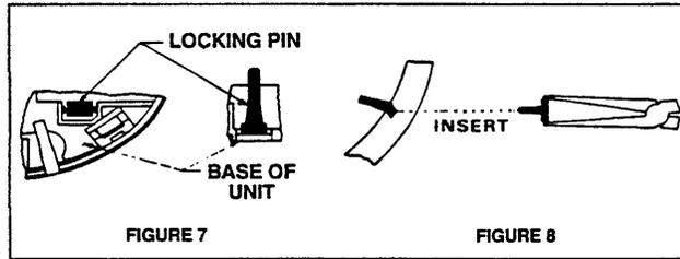
To make the smoke alarm somewhat tamper resistant, a "locking pin" has been provided in the base of the unit. It will help deter a child or other individual from removing the smoke alarm from the bracket. See Figure 7. The following directions can install this.
