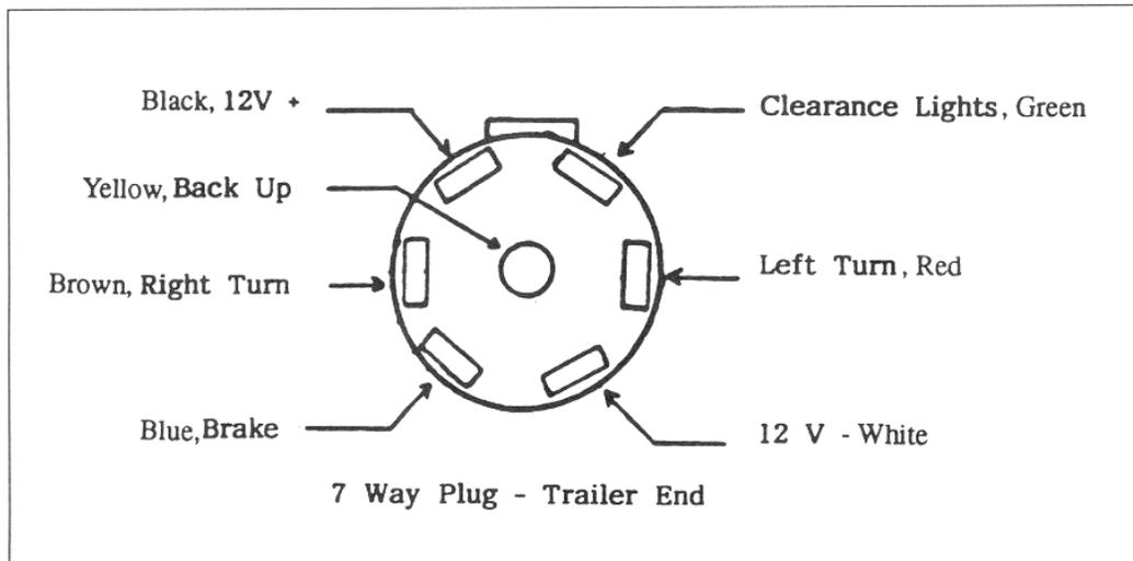
**Note:** The 7 way wire is spliced to the main harness behind the front sofa in the front of the trailer.
