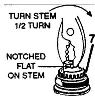
1. Remove plug button (3) from the handle by prying the button upwards from the bottom center. If a tool is required, use something, which will not scratch the handle. Remove set-screw (2), handle body (1), dome and pivot retainer assembly (4), cartridge screw (5), handle adapter and handle connector assembly (6).
