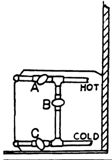
Open the hot side of the galley or lavatory faucet and turn on the water pump switch located on the monitor panel. For some time the open faucet will only sputter. This is because the water heater is being filled and air is being pushed out through the lines. Once the water heater is full a steady stream of water will come from the faucet. Now open a cold faucet. It will sputter for a short time, but will soon expel a steady stream. All other faucets can now be opened until all air is expelled.
