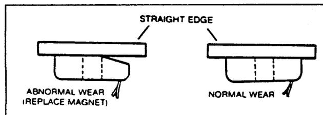
Even if wear is normal is indicated by your straightedge the magnets should be replaced if any part of the magnet coil has become visible through the friction material facing of the magnet. It is also recommended that the drum armature surface be re-faced when replacing magnets. (See Brake Drum Section) Magnets should also be replaced in pairs (both sides of an axle). Use only genuine Dexter replacement parts when replacing your magnets.
