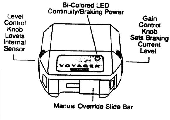
**ELECTRONIC CONTROLLERS** are inertially activated. The controller senses deceleration and generates an output, which reflects the inertia sensed. When your stationary, the controller does not apply the brakes unless the manual slide bar is activated.
