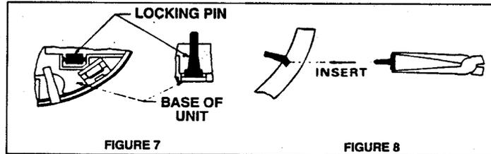
3. Using long-nose pliers grab the head of the locking pin and insert into hole located on the side of the smoke alarm. See Figure 8.
